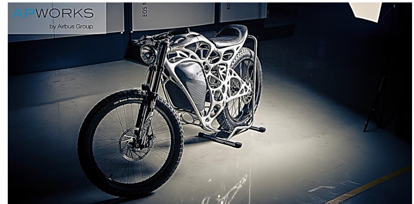
Quelle: Airbus APWorks, Light Rider, -30% Gewicht (35kg)
